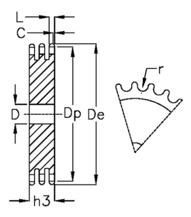
C = 2 D = 30 De = 494.2 Dp = 485.22 For chain size =  $3/4 \times 7/16$ For chain type = 12 B-3 h3 = 49.8 L = 10.8 Number of teeth = 80r = 12.07
